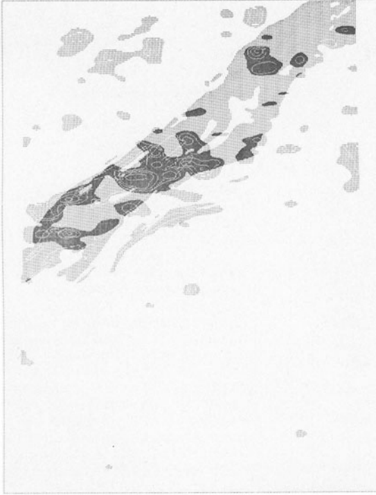
Figure 4. Coincidence (black areas) between EU/ETH highs ( >0.20 , horizontal lines) and aeromagnetic anomaly lows ( <2100 gammas, vertical lines). The two geophysical-anomaly image-sets are identified as A1 and A2 in the text and in Figure 7. EU/ETH is the ratio of equivalent uranium to equivalent thorium concentrations detected by low flying aircraft.
